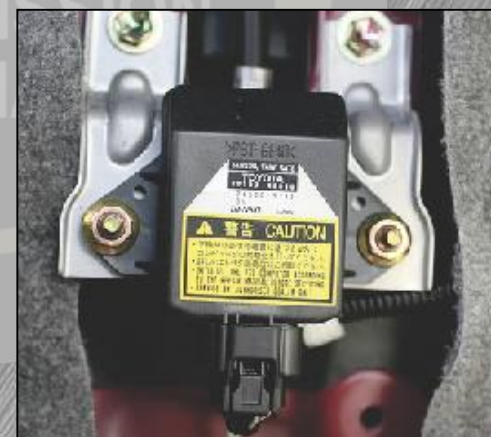
Typical External Type G (Yaw) Sensor
