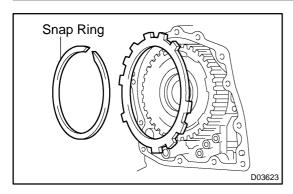
(c) Temporarily remove the snap ring, attach the selected flange and restore the snap ring.
