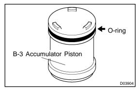
(b) Remove the O-ring from the B-3 accumulator piston.
