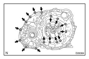
(f) Remove the 16 bolts and the transaxle housing.
