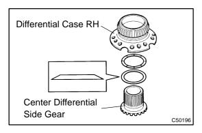
(d) Remove the center differential side gear, conical spring washer and center differential side gear thrust washer No.1 RH from the differential case RH.
