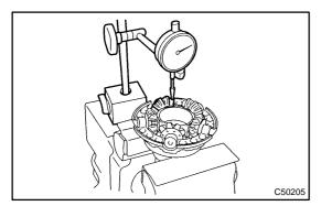
(c) Pressing and holding the differential spider toward the differential case RH, measure the pinion's backlash with a dial indicator as illustrated.
