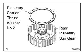
(c) Remove the planetary carrier thrust washer No.2 from the rear planetary sun gear assy.
