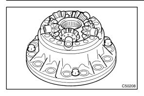
(f) Remove the differential spider, 5 center differential pinions and 5 center differential pinion thrust washers from the differential case RH. Put them in the differential intermediate case and fix the case.
