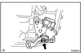
(i) Install the control shaft lever, washer and nut.
