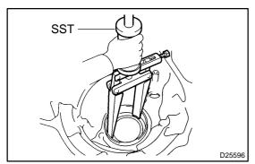
(b) Using SST, remove the front differential case front tapered roller bearing outer race and differential case washer.
