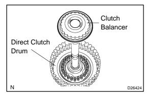
(c) Remove the clutch balancer from the direct clutch drum.
