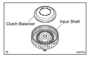
(c) Install the clutch balancer to the input shaft.
