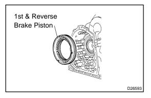
(c) Coat a 1st & reverse brake piston with ATF, install it to the transaxle case.
