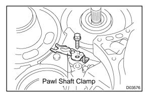
(c) Install the pawl shaft clamp with the bolt.
