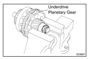
(b) Clamp the underdrive planetary gear in soft jaw vise.
