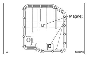
(b) Remove the 2 magnets from the oil pan.
