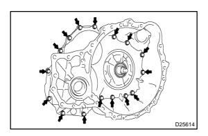
(g) Remove the 16 bolts and the transaxle housing.
