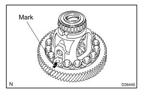
(c) Align the match-marks, install the front differential ring gear case quickly.
