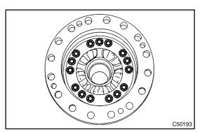
(I) Install the adjusted differential case RH to the intermediate case and tighten the 15 bolts using a torx socket wrench (T50).
