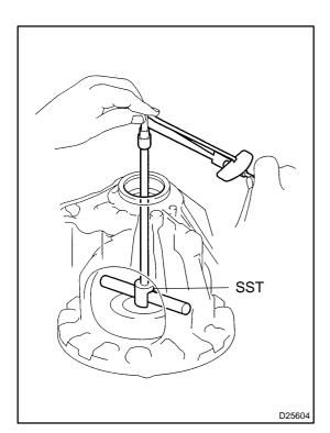
(d) Using SST, turn the differential assy right and left 2 or 3 times to settle the bearing.
