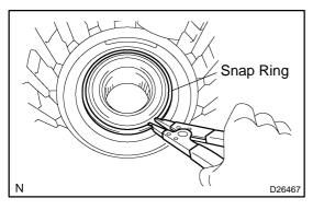
(c) Using a snap ring expander, install the snap ring.
