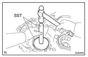
(b) Using SST and a hammer, install the front differential case tapered roller bearing front outer race to the transaxle housing.
