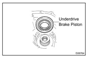
(c) Install the underdrive brake piston to the transaxle case. **NOTICE:**
