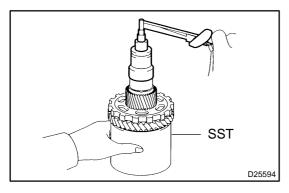
(b) Using SST and a torque wrench, measure the turning torque of underdrive planetary gear assy while rotating the torque wrench at 60 rpm.
