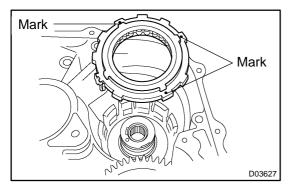
(b) Install the 1-way clutch to the transaxle case.
