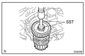
(c) Using SST and a press, remove the front planetary gear assy from the counter drive gear.
