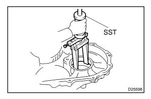
(b) Using SST, remove the front differential case rear tapered roller bearing outer race.
