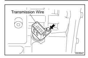
(b) Install the transmission wire retaining bolt. Torque: 5.4 N·m (55 kgf·cm, 48 in. lbf)
