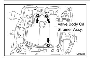
(b) Install the oil strainer and 3 bolts to the valve body. Torque: 11 N·m (110 kgf·cm, 8 ft·lbf)
