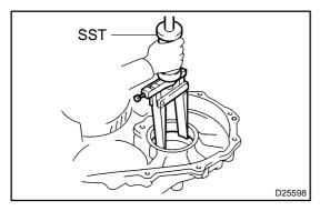
(b) Using SST, remove the front differential case rear tapered roller bearing outer race and differential case washer.
