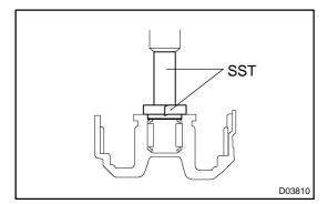
(c) Using SST and a press, install the needle-roller bearing to the transaxle case.
