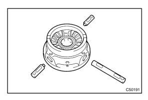
(f) Remove the center differential pinion shaft and 2 differential pinion shafts.
