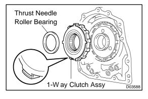
(c) Install the 1-way clutch and thrust needle roller bearing to the 1-way clutch sleeve outer.
