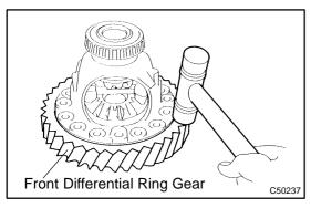
(c) Using a plastic hammer, tap on the front differential ring gear to remove it from the case.
