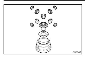
(g) Remove 4 front differential pinions, 4 front differential pinion thrust washers, front differential pinion shaft holder, front differential planetary ring gear and differential side gear thrust washer No. 1.
