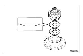
(d) Temporarily install the differential side gear thrust washer No.2 LH, center differential side gear conical spring washer and differential case No.2 to the differential case LH.
