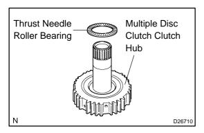
(b) Coat the thrust needle roller bearing and race with yellow petrolatum, install them onto the multiple disc clutch hub.
