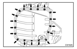
(c) Install the new oil pan gasket with the 18 bolts to the transaxle case.
