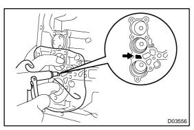
(b) Apply compressed air (392 kPa, 4.0 kgf/cm<sup>2</sup>, 57 psi) to the oil hole and remove the C-3 accumulator piston.
