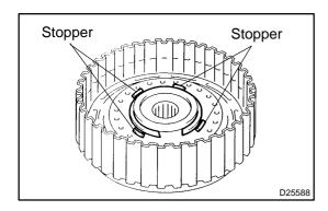
(g) Set the end gap of the snap ring in the piston shown in the illustration.
