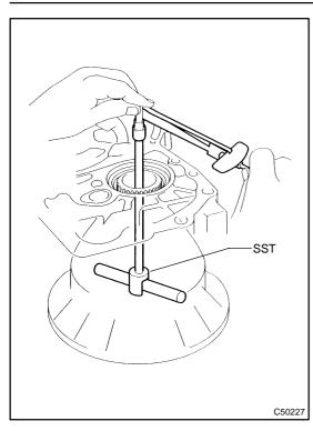
(e) Using SST, turn the differential assy right and left 2or 3 times to allow the bearing settle.
