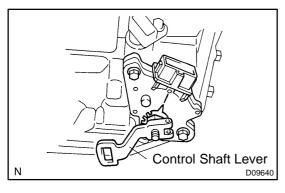
(c) Temporarily install control shaft lever.
