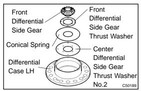
(c) Remove the front differential side gear, front differential side gear thrust washer, conical spring and center differential side gear thrust washer No.2 from the differential case LH.
