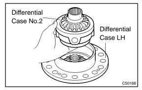
(k) Install the differential case No. 2 to the differential case LH again.
