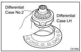
(i) Remove the differential case No.2 from the differential case LH.
