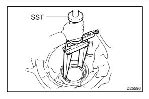
(b) Using SST, remove the front differential case front tapered roller bearing outer race.
