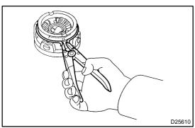
(h) Using a snap ring expander, install the pinion shaft spacer snap ring.
