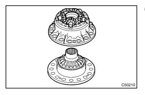
(h) Remove the 4 bolts and disconnect the differential case LH from the differential intermediate case.
