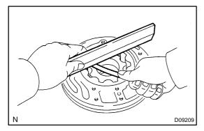
(d) Using a straight edge and feeler gauge, measure the side clearance of both gears.
