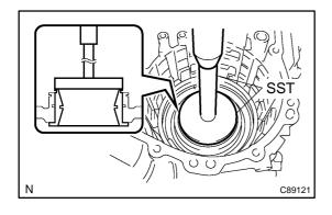
(b) Using SST and a press, remove the bearing outer race. SST 09950-60020 (09951-00910), 09950-70010 (09951-07100)
