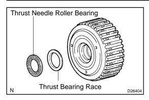
(b) Remove the thrust needle roller bearing and thrust bearing race from the rear planetary sun gear assy.
