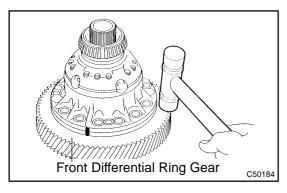
(c) Using a plastic hammer, tap on the ring gear to remove it from the case.
