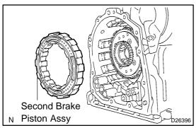
(b) Remove the second brake piston assy from the transaxle case.
