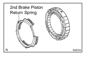
(c) Remove the 2nd brake piston return spring.
