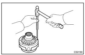
(e) Using a pin punch and a hammer, remove 3 straight pins.
