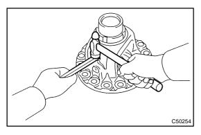
(b) Using a chisel and hammer, stake the differential case.
