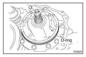
(b) Coat the O-ring of oil pump with ATF.
