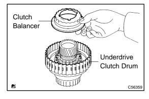
(c) Install the clutch balancer to the underdrive clutch drum. **NOTICE**:
