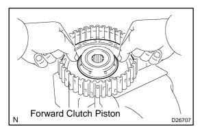
9. INSTALL FORWARD CLUTCH PISTON SUB-ASSY
