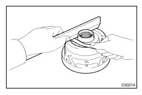
(f) Using a straight edge and feeler gauge, measure the clearance between the front differential case and the front differential side gear.
