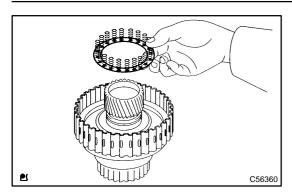
(d) Remove the return spring from the underdrive clutch drum.
