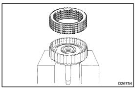
(b) Remove the flange, 5 discs and 5 plates from the input shaft assy.
