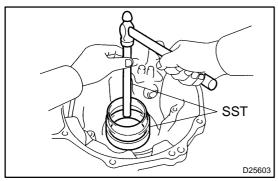
(b) Using SST, install the outer race of the tapered roller bearing FR.
