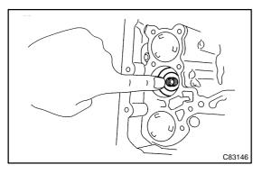
Coat the piston with ATF, install it to the transaxle case. (b) NOTICE:
