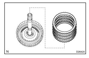
(b) Remove the flange, 3 discs,, 3 plates and cushion plate from the intermediate shaft.
