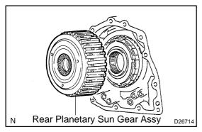
(c) Install the rear planetary sun gear assy to the rear planetary gear.
