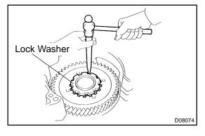
(g) Using a chisel and hammer, stake the front lock washer.
