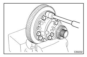
(d) Temporarily install the 8 bolts as shown in the illustration.
