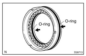
(b) Remove the 2 O-rings from the 1st & reverse brake piston.
