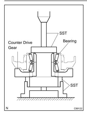
(c) Using SST and a press, install the counter drive gear and bearing to the transaxle case.
