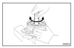
clutch assy after inserting the multiple disc clutch into it.  $\mbox{\bf NOTICE:}$
