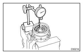
(b) Using a dial indicator, measure the backlash of one pinion gear while holding the front differential side gear toward the case.
