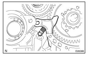
(b) Temporarily install the parking lock pawl, shaft and spring to the transaxle case, as shown in the illustration.
