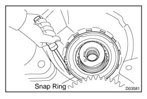
(c) Using a screwdriver, install the snap ring to the transaxle case.
