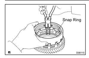
(e) Using a snap ring pliers, install the snap ring.
