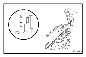
(d) Using a straight edge and vernier calipers as shown in the illustration, measure the gap between the top of the differential drive pinion in the underdrive planetary gear and contact surface of the transaxle case and housing (Dimension E).
