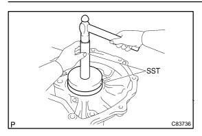
(b) Using SST and a hammer, install the front differential case tapered roller bearing front outer race to the transaxle housing.
