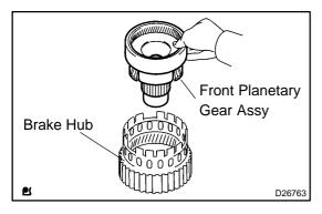
(d) Remove the front planetary gear assy from the brake hub.
