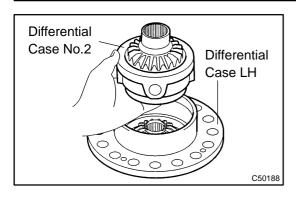
(b) Remove the differential case No.2 from the differential case LH.
