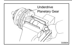
(c) Using a socket wrench, remove the lock nut.
