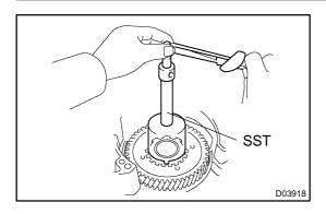
(e) Using SST and a torque wrench, measure the turning torque of the bearing while rotating SST at 60 rpm. When the measured value is not within the specified value, gradually tighten the nut until it reaches the specified value.
