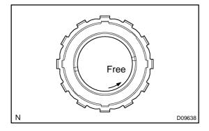
(b) Check the rotating direction of 1-way clutch for the lock or free operation, as shown in the illustration.
