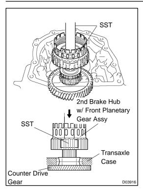
(b) Using SST and a press, press-fit the front planetary gear assy.
