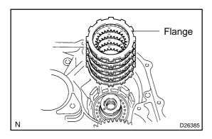
(b) Remove the flange, 4 discs and 4 plates from the transaxle case.
