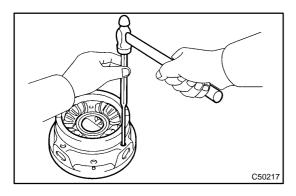
(g) Using a pin punch and a hammer, install 3 straight pins.
