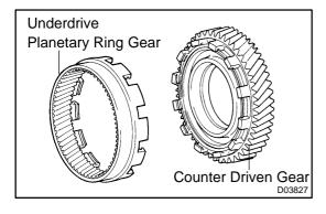
(d) Install the underdrive planetary ring gear to the counter driven gear.
