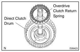
(d) Remove the overdrive clutch return spring from the direct clutch drum.
