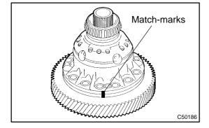
(c) Set the match-marks, install the front differential ring gear case quickly.
