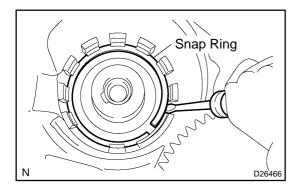
(c) Using a screwdriver, install the snap ring.
