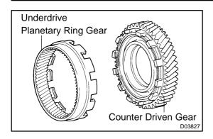
(b) Remove the underdrive planetary ring gear from the counter driven gear.
