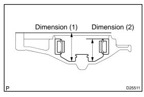
(e) As shown in the illustration, measure the 2 places of the transaxle housing, calculate the dimension F using the formula.
