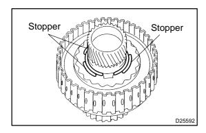
(g) Set the end gap of the snap ring in the underdrive clutch drum shown in the illustration.
