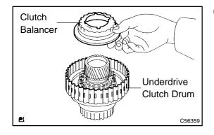
(c) Remove the clutch balancer from the underdrive clutch drum.
