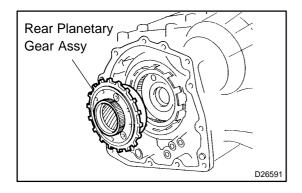
(b) Remove the rear planetary gear assy from the transaxle case.
