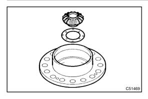
(j) Install the selected differential side gear thrust washer No. 2 LH and center differential planetary gear to the differential case LH.
