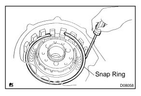
(b) Install the snap ring and measure the inside diameter.
