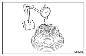
(g) Pressing and holding the differential spider toward the differential intermediate case, measure the pinion's backlash with a dial indicator.
