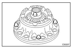
(e) Install the differential intermediate case to the above and fix them with 4 bolts.
