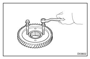
(b) As shown in the illustration, tighten 2 bolts evenly and make clearance of approx. 20.0 mm (0.797 in.) between the counter drive gear and the inner race.
