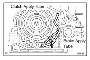
(c) Install the brake apply tube and a bolt to the transaxle case.
