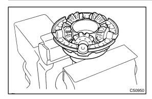
(b) Hold the differential case RH by vice. Install the center differential pinion and pinion thrust washer to the differential spider and install them to the differential case RH.
