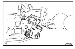
(h) Using a screwdriver, stake the nut with the nut stopper.
