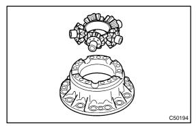
(e) Remove the differential spider, 5 center differential pinions and 5 center differential pinion thrust washers from the differential intermediate case.
