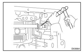
(b) Using a pin punch and hammer, drive in a new pin.
