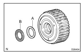
(b) Coat the bearing with yellow petrolatum, install it onto the rear planetary sun gear.
