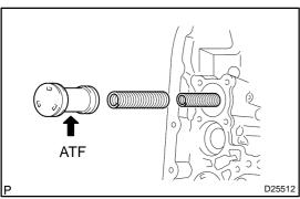
(b) Coat the piston with ATF, install it to the transaxle case. **NOTICE:**
