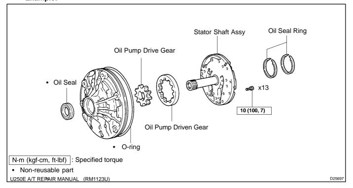
(d) Tightening torque, oil applying position, and non-reusable parts are described as important points in the procedure.
