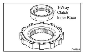
(b) Remove the 1-way clutch inner race from the 1-way clutch assy.
