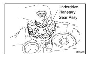
(d) Remove the underdrive planetary gear assy from the transaxle case.
