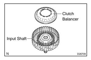
(c) Remove the clutch balancer from the input shaft.
