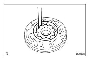
(c) Using a feeler gauge measure the tip clearance between the driven gear teeth and drive gear teeth.
