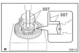
(c) Using SST and a press, press in the outer race of the tapered roller bearing.
