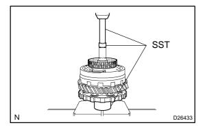
(d) Using a press, press in the parking lock gear. SST 09502-12010, 09950-60010 (09951-00260), 09950-70010 (09951-07100), 09316-20011
