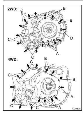
(c) Install the transaxle housing and 16 bolts to the transaxle case.
