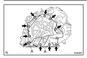
(c) Apply liquid sealer to the "A" bolt threads.
