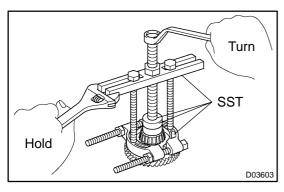
(c) Using SST, remove the tapered roller bearing. SST 09950-60010 (09951-00590), 09950-70010 (09951-07100), 09950-00020, 09950-00030, 09950-4001 1 (09957-04010)
