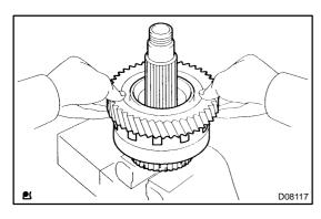
(b) Install the counter driven gear with planetary ring gear to the underdrive planetary gear.
