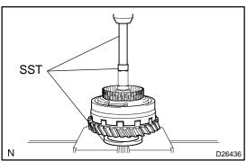
(c) Using SST and a press, press in the front tapered roller bearing.
