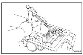
(b) Using a pin punch and hammer, drive out the spring pin. HINT:
