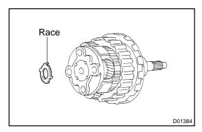
(d) Coat the race with petroleum jelly and install it onto the O/D planetary gear.
