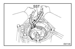
(e) Using SST, install the snap ring. SST 09350-30020 (09350-07060)
