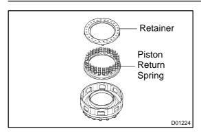
(c) Remove the retainer and piston return spring.
