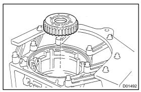
(c) Install the No. 1 one-way clutch to the multiple disc brake.
