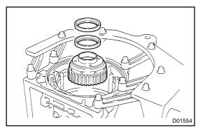
(e) Install the front planetary gear and 2 washers from the case.
