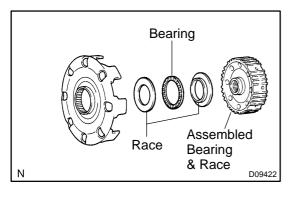
(b) Remove the assembled bearing & race, 2 races, bearing and sun gear input drum, from forward clutch hub.
