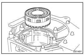
(d) Remove the multiple disc brake from the case.
