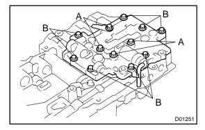
(d) Install the 12 bolts. 2 of them are attached to the oil cooler pipe and clamp. So install them all together.
