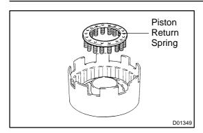
(c) Remove the piston return spring.
