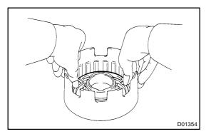
(b) Being careful not to damage the O-rings press in the direct clutch piston into the clutch drum with both hands.
