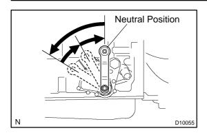
(c) Using the control shaft lever, fully turn the manual lever shaft back and return 2 notches. It is now in neutral.
