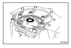
(d) Remove the assembled bearing & race from the case.
