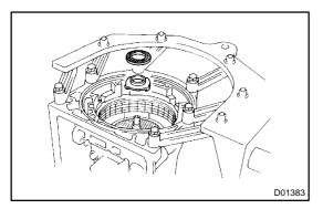
(c) Install the bearing and race onto the O/D planetary ring gear.
