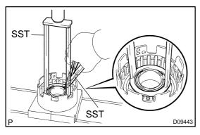
(b) Place SST on the spring retainer, and compress the return spring with a press.
