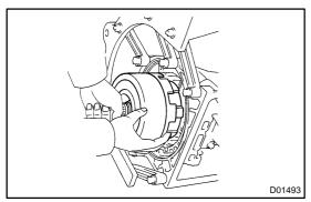
(d) Insert the direct clutch with forward clutch to the case.
