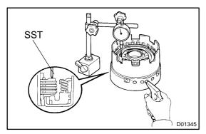
(b) Using SST and a dial indicator, measure the direct clutch piston stroke while applying and releasing compressed air (186 - 206 kPa, 1.9 - 2.1 kgf/cm<sup>2</sup>, 27 - 30 psi).
