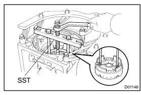
(c) Using SST, remove the O/D support assembly. SST 09350-30020 (09350-07020)
