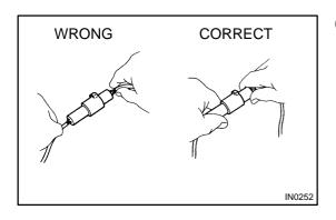
(j) To pull apart electrical connectors, pull the connector itself, not the wires.
