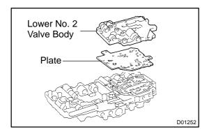
(c) Align the holes of lower No. 2 valve body with those of plate and place them on the lower No. 1 valve body with aligning all the holes.
