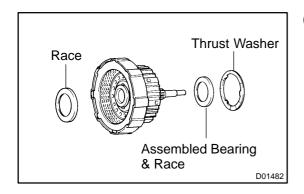
(c) Remove the assembled bearing & race, thrust washer and race from the forward clutch.
