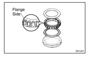
(b) Install the one-way clutch and 2 inner races into the outer race with the flange side of the one-way clutch facing upward.
