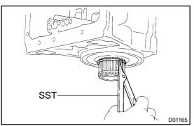
Using SST, install the snap ring. (c) SST 09350-30020 (09350-07070)
