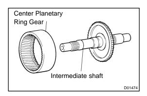
(b) Remove the center planetary ring gear from the intermediate shaft.
