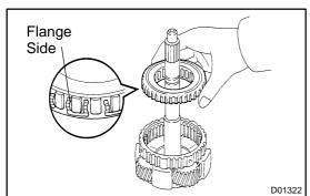
(c) Install the O/D one-way clutch with the outer race to the O/D planetary gear.
