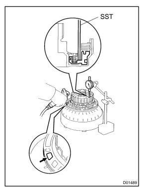
(b) Using SST and a dial indicator, measure the O/D direct clutch piston stroke while applying and releasing compressed air (392 kPa, 4 kgf/cm², 57 psi).
