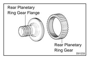
(b) Remove the rear planetary ring gear flange from the rear planetary ring gear.
