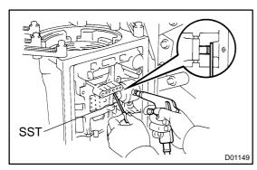
(b) Using SST, measure the stroke while applying and releasing compressed air (392 kPa, 4 kgf/cm<sup>2</sup>, 57 psi).
