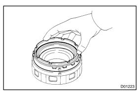
(c) Being careful not to damage the O-rings, press the 2nd brake piston into the brake drum with both hands.
