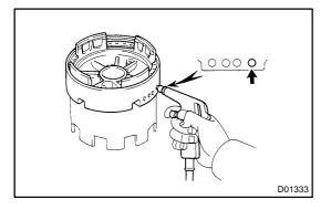
(b) Apply compressed air (392 kPa, 4 kgf/cm<sup>2</sup>, 57 psi) into the oil passage and be sure that the O/D brake piston moves smoothly.
