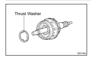
(b) Install the thrust washer to the output shaft with center & rear planetary gear.
