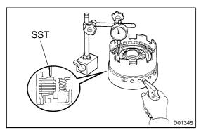
(b) Using SST and a dial indicator, measure the direct clutch piston stroke while applying and releasing compressed air (186 kPa, 1.9 kgf/cm<sup>2</sup>, 27 psi).
