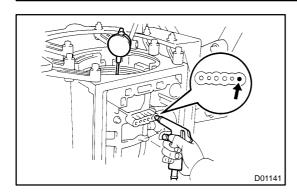
(b) Measure the stroke while applying and releasing compressed air (392 kPa, 4 kgf/cm², 57 psi).
