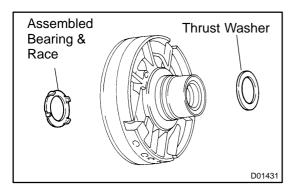
(d) Remove the assembled bearing & race and thrust washer from the O/D support.
