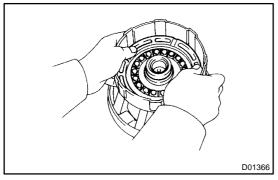
(b) Being careful not to damage the O-rings, press the clutch piston into the forward clutch drum with both hands.
