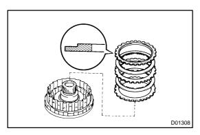
(b) Remove the flange, 2 plates and 2 discs.
