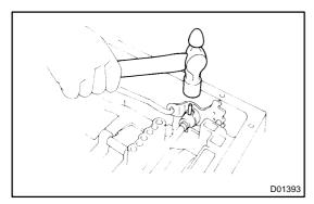
(e) Using a hammer, drive in a new spring pin.
