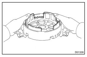
(b) Being careful not to damage the O-rings, press in the brake piston into the O/D support with both hands.
