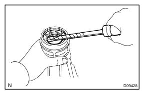
2. REMOVE EXTENSION HOUSING OIL SEAL Using a screwdriver, remove the oil seal.
