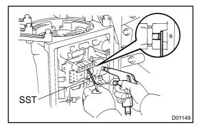
(b) Using SST, measure the stroke while applying compressed air (392 kPa, 4 kgf/cm², 57 psi). SST 09240-00020
