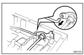
(b) Disconnect the parking lock rod from the manual valve lever.
