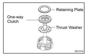
(b) Remove the retaining plate, one-way clutch and thrust washer.
