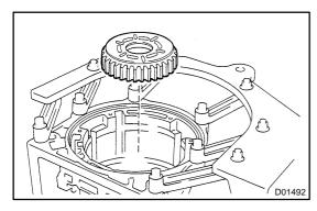
(b) Remove the No. 1 one-way clutch from the case.
