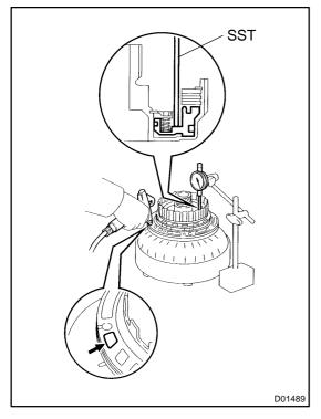
(b) Using SST and a dial indicator, measure the O/D direct clutch piston stroke while applying and releasing compressed air (392 kPa, 4 kgf/cm², 57 psi).
