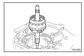
(c) Remove the output shaft with center & rear planetary gear from the case.
