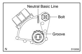
(d) Align the neutral basic line with the switch groove, and tighten the adjusting bolt.
