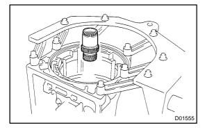
Install the front & center planetary sun gear from the case. (c)
