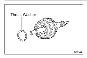
(d) Remove the thrust washer from the output shaft with center & rear planetary gear.
