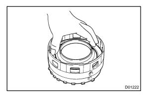
(b) Being careful not to damage the O-rings, press the 3rd brake piston into the brake drum with both hands.
