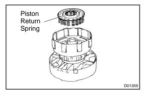
(c) Remove the piston return spring.
