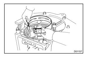
(d) Remove the 3rd coast brake band from the case.
