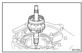
(c) Install the output shaft with center & rear planetary gear.
