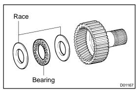
(c) Remove the assembled bearing & race and 2 races from the rear planetary ring gear.
