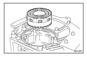
(b) Install the multiple disc brake to the case.
