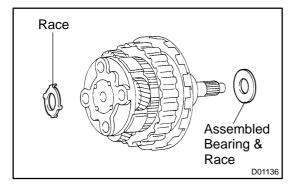
(b) Remove the race and assembled bearing & race.
