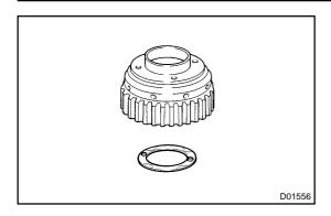
(d) Coat the thrust washer, with petroleum jelly and install it onto front planetary gear.
