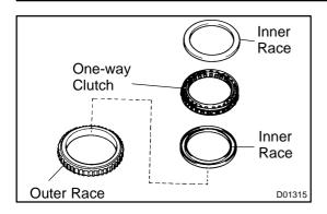
**9. REMOVE ONE-WAY CLUTCH FROM OUTER RACE** Remove the 2 inner races and one-way clutch to the outer race.
