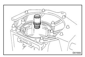
(g) Remove the front & center planetary sun gear from the case.
