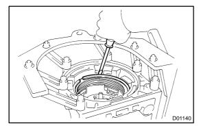
(e) Using a screwdriver, install the snap ring.
