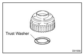
(f) Remove the thrust washer from the front planetary gear.
