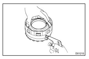
(b) Hold the 3rd brake piston so that it dose not slant, and apply compressed air (392 kPa, 4 kg/cm², 57 psi) into the passage to remove the 3rd brake piston.
