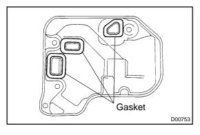
(c) Remove the 3 gaskets from the oil strainer.
