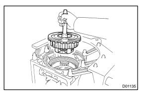
(e) Install the O/D planetary gear with the O/D direct clutch & O/D one-way clutch.
