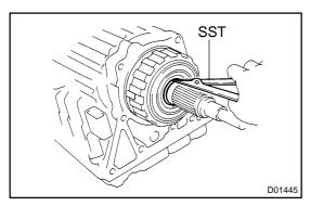
(b) Using SST, install the snap ring. SST 09350-30020 (09350-07070)
