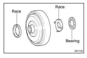
(b) Remove the bearing and 2 races from the planetary ring gear.
