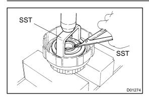
(b) Place SST on the spring retainer, and compress the return spring with a press.
