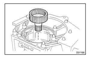
(b) Remove the rear planetary ring gear from the case.
