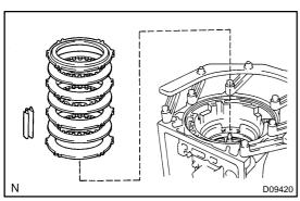
(b) Remove the O/D brake pack as a set. HINT:
