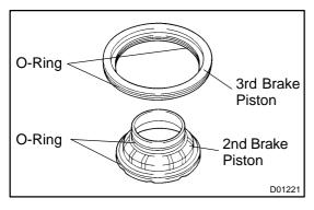
(c) Remove the 4 O-rings from the 3rd and 2nd brake pistons.
