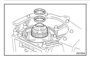
(e) Remove the 2 washers and front planetary gear from the case.
