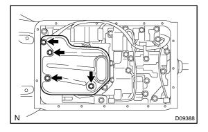
(b) Install the oil strainer with the 4 bolts.
