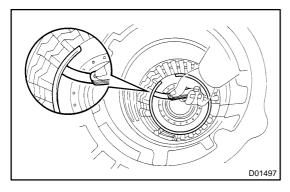
(b) Using feeler gauge, measure 1st & reverse brake pack clearance between the snap ring and the flange.
