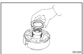
2. REMOVE CLUTCH DRUM THRUST WASHER FROM O/D SUPPORT
