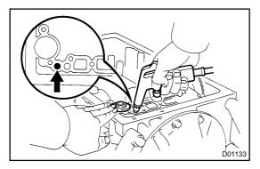
(e) Applying compressed air to the oil hole, remove the C<sub>0</sub> accumulator piston and spring.
