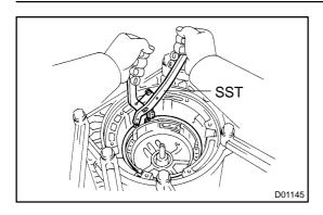
(b) Using SST, remove the snap ring. SST 09350-30020 (09350-07060)
