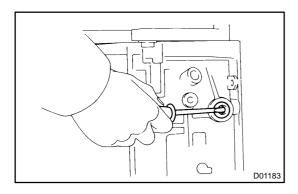
(d) Using a screwdriver, remove the 2 oil seals.
