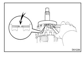
(c) Assemble the snap ring to the front planetary ring gear. Nip the both ends of snap ring using needle nose pliers and install them to the output shaft with rear planetary gear so that the end gap of the snap ring comes on the indented part of the output shaft with rear planetary gear.
