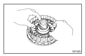
(b) Being careful not to damage the O-rings, press the direct clutch piston into the clutch drum with both hands.
