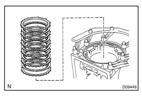
(b) Remove the flange, 5 discs and 5 plates.
