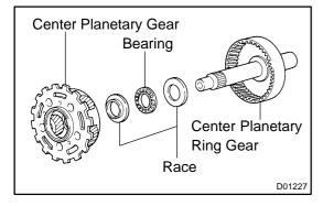
(b) Remove the center planetary gear, bearing and 2 races from center planetary ring gear.
