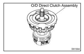
2. REMOVE O/D DIRECT CLUTCH ASSEMBLY FROM O/D PLANETARY GEAR
