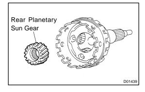
2. INSTALL REAR PLANETARY SUN GEAR
