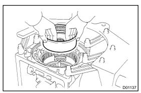
(b) Install the O/D planetary ring gear.
