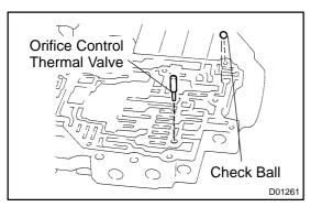
(e) Remove the orifice control thermal valve and check ball.
