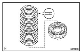
(b) Remove the flange, 7 plates and 4 discs.
