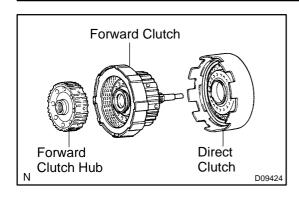
(c) Install the direct clutch and forward clutch hub to the forward clutch.
