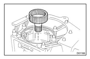
(b) Install the rear planetary ring gear.
