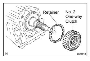
(b) Remove the No. 2 one-way clutch and the retainer.
