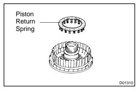
(c) Remove the piston return spring.
