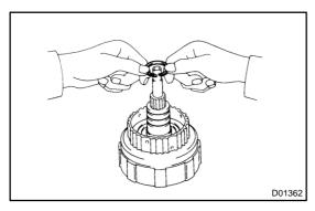
7. REMOVE 3 OIL SEAL RINGS FROM FORWARD CLUTCH
