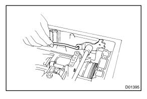
(c) Connect the parking lock rod to the manual valve lever.
