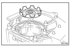
(b) Install the sun gear input drum.
