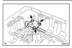
(d) Place the parking lock pawl bracket onto the transmission case and torque the 3 bolts.
