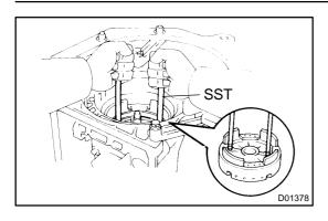
(c) Using 2 bolts of SST, face the bolt and oil holes of the O/D support toward the valve body side, align them with the bolt holes of the transmission case and install the bolts. SST 09350-30020 (09350-07020)
