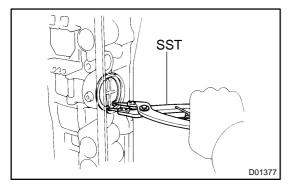
(c) Using SST, install the snap ring. SST 09350-30020 (09350-07060)
