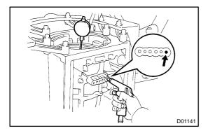
(b) Measure the stroke while applying and releasing compressed air (392 kPa, 4 kgf/cm<sup>2</sup>, 57 psi).
