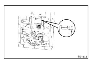
(e) With the case set upright, using vernier calipers, measure the distance between the sun gear input drum and direct clutch drum.
