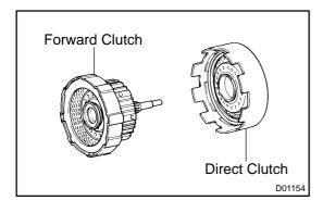
(b) Remove the direct clutch from the forward clutch.
