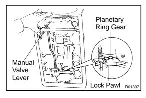
(e) Shift the manual valve lever to the P position, and confirm the planetary ring gear is correctly locked up by the lock pawl.
