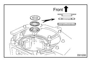
(c) Coat the bearing, 2 races with petroleum jelly and install them onto the sun gear input drum.
