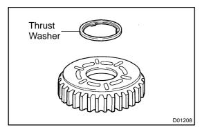
(c) Remove the thrust washer from the No. 1 one-way clutch.
