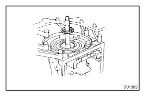
(f) Install the assembled bearing & race onto the O/D direct clutch.
