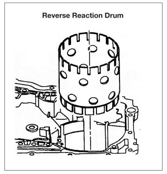
Note design change of reverse reaction drum. This also affects the 2nd clutch drum as well as the input carrier.
