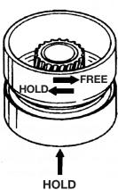
Must rotate counterclockwise and hold clockwise.
