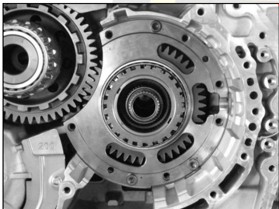
Output Speed Sensor (OSS) Monitors Transfer Drive Gear
