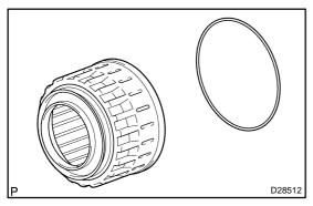
(b) Remove the O-ring from the reverse clutch piston sub assy.
