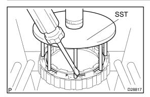
(c) Using SST and press, install the snap ring. **NOTICE:**
