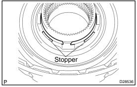
(f) Set the end gap of the snap ring in the piston as shown in the illustration.
