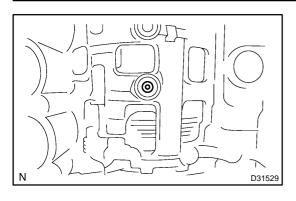
(d) Check that the oil pressure apply hole of the brake cylinder No.2 aligns with the oil pressure apply hole of the transmission case.
