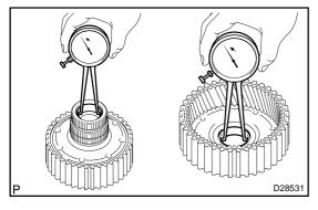
63. INSPECT RR PLANETARY RING GEAR FLANGE SUB-ASSY
