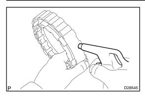
(c) Hold the 2nd brake piston and apply compressed air (392 kPa, 4.0 kgf/cm², 57 psi) to the 2nd brake cylinder to remove the 2nd brake piston.
