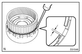
Using a screwdriver, install the snap ring. (b)
