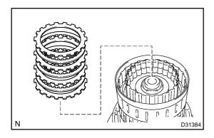
(b) Remove the flange, the 3 discs and the 3 plates from the input shaft assy.
