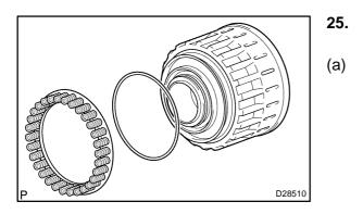
25. REMOVE REVERSE CLUTCH RETURN SPRING SUB-ASSY
