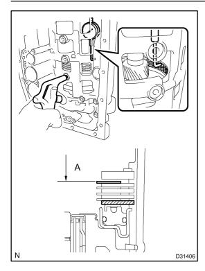
(b) Using a SST and a dial gauge, measure the moving distance (distance A) of the clutch disc at the both ends across a diameter while blowing air from the oil hole as shown in the illustration, and calculate the average. SST 09350-30020 (09350-06120)
