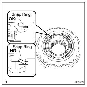
(c) Set the end gap of the snap ring in the piston as shown in the illustration.
