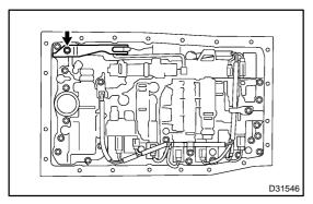
(c) Install the detente spring with the bolt.
