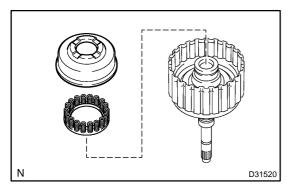
(c) Remove the clutch balancer No.1 and the forward clutch return spring from the input shaft assy.
