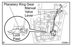
(b) Shift the manual valve lever to the P position, and confirm the planetary ring gear is correctly locked up by the lock pawl.
