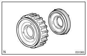
(b) Remove the coast clutch piston from the forward clutch piston.
