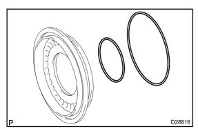
(d) Remove the 2 O-rings from the direct clutch piston subassy.
