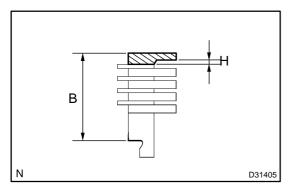
(c) Using vernier calipers, measure the thickness (length B) of the brake flanges the 4 brake plates No.4 and the 4 brake discs No.4 altogether at the both ends across a diameter, and calculate the average.
