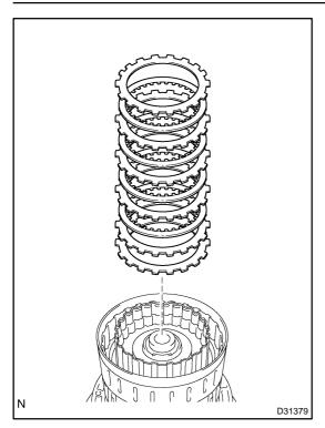
(b) Remove the flange, cushion plate, 4 discs and 4 plates from the input shaft assy.
