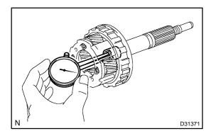
(b) Using a dial indicator, measure the inside diameter of the rear planetary gear bushing.
