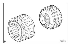
(c) Be careful not to damage the O-ring. Press in the clutch drum sub assy into the reverse clutch piston with both hands.
