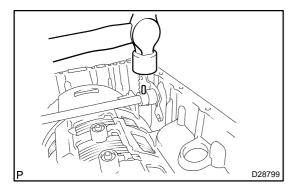
(c) Using a hammer, drive in a new spring pin.
