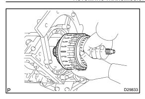
(c) Install the input shaft sub assy with the clutch drum &input shaft assy onto the transmission case.
