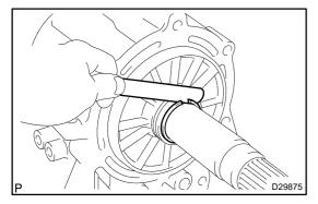
(c) Using feeler gauge, measure the clearance between the snap ring and the race.
