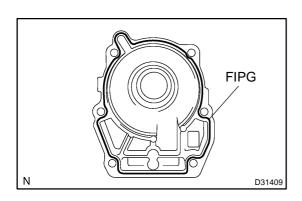
(e) Apply FIPG to the extension housing as shown in the illustration.
