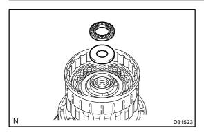
(c) Remove the thrust needle roller bearing and thrust bearing race from the clutch drum assy.
