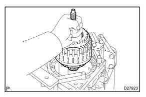
31. REMOVE CLUTCH DRUM & INPUT SHAFT ASSY
