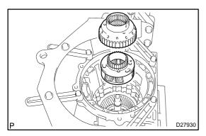
(c) Install the front planetary gear assy and the 1 way clutch inner race to the case.
