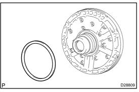
(c) Remove the thrust bearing race No.1 from the oil pump.
