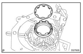
50. REMOVE BRAKE PISTON RETURN SPRING SUB-ASSY
