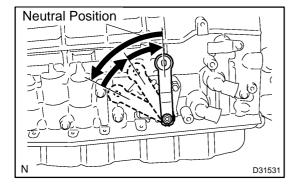
(c) Using the control shaft lever, turn the manual lever shaft back all the way and then forward 2 notches. It is now in neutral.
