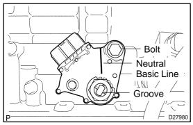
(d) Align the neutral basic line with the switch groove as shown in the illustration, and tighten the adjusting bolt.
