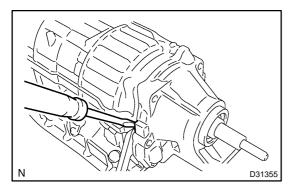
(d) Use a screwdriver to remove the extension housing subassy.
