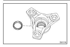
(c) Remove the oil seal from the flange yoke assy.
