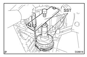
(b) Using SST and a press, install the brake No.2 spring snap ring.
