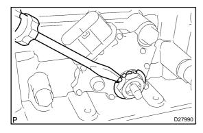
(e) Using a screwdriver, bend the tabs of the lock washer. HINT:
