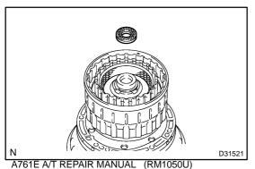
(b) Install the thrust needle roller bearing to the clutch drum assy.
