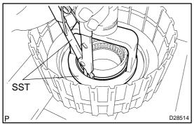
28. REMOVE DIRECT CLUTCH PISTON SUB-ASSY
