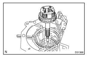
(b) Remove the thrust bearing race No.9 and the thrust needle roller bearing from the rear planetary gear assy.
