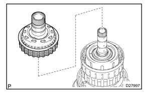
(b) Remove the reverse clutch hub sub assy with the reverse clutch reaction sleeve, the clutch cushion plate, the reverse clutch flange, the 5 reverse clutch discs, and the 4 clutch plates from the clutch drum assy.
