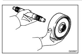
Remove the ring gear and flange assembly from (b) the intermediate shaft.
