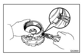
**REMOVE FRONT PLANETARY RING GEAR** 11. Using needle nose pliers, pry out the ring gear while compressing the snap ring.
