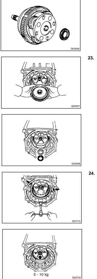
(d) Remove the bearing from the O/D planetary gear or ring gear flange.
