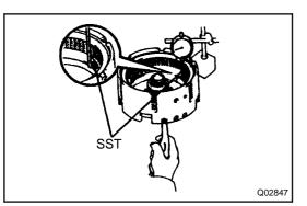
3. CHECK PISTON STROKE OF SECOND BRAKE
