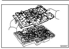
(c) Remove the lower valve body together with the valve body
