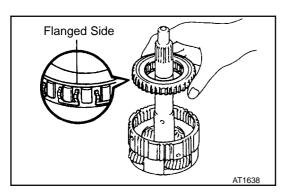
(b) Install the one-way clutch and 2 retainers into the outer race.
