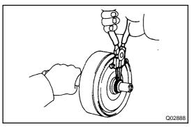
(b) Install the ring gear and flange assembly.
