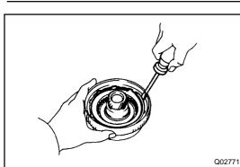
Using a screwdriver, install the snap ring.
