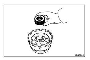
7. INSTALL REAR PLANETARY SUN GEAR Install the sun gear to the rear planetary gear.
