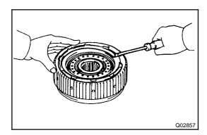
2. INSTALL NO. 2 THRUST WASHER Coat the thrust washer with petroleum jelly, and install it onto the rear planetary gear.
