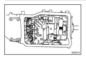
Disconnect the 4 connectors from the solenoids. (b)
