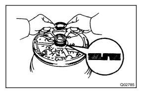
2. REMOVE OIL SEAL RINGS Remove the 2 oil seal rings. AUTOMATIC TRANSMISSION - OIL PUMP
