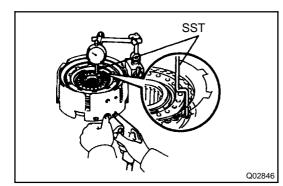
Using SST and a dial indicator, measure the piston stoke while applying and releasing compressed air 392 - 785 kPa (4 - 8 kgf/cm<sup>2</sup>, 57 - 114 psi).
