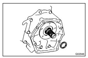
(b) Using snap ring pliers, remove the snap ring.
