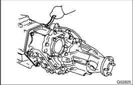
**39. INSTALL TRANSFER ASSEMBLY** Install the transfer assembly with 6 bolts.
