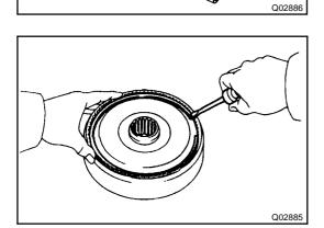
**REMOVE REAR PLANETARY RING GEAR FLANGE** 10. Using a small screwdriver, remove the snap ring. (a)
