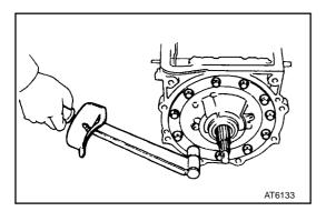
(d) Install and tighten the 11 bolts. Torque: 21 N-m (210 kgf-cm, 16 ft-lbf)
