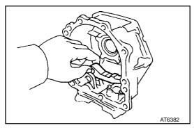
(b) Using SST and calipers, set the pawl bracket so that the distance between the transfer adaptor surface and the top of the bracket tab is the specified distance.
