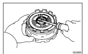
12. REMOVE NO. 2 THRUST WASHER Remove the thrust washer from the rear planetary
