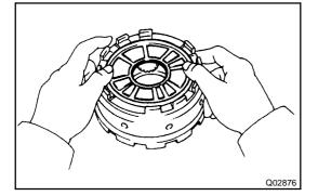
HINT: Securely fit the lips of the thrust washer into the holes of the rear planetary gear.
