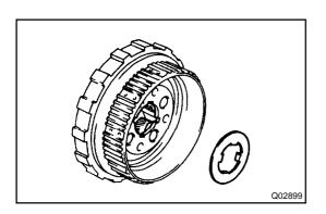
(d) Using a screwdriver, install the snap ring. HINT: Be sure the end gap of the snap ring is not aligned with the cutout portion of the rear planetary gear.
