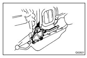
(b) Remove the nut, lock washer and grommet.
