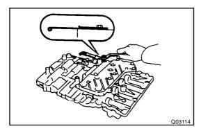
(b) Install the body cover with the 2 wave washers and 14 bolts.
