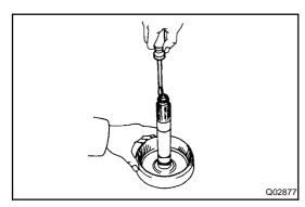
8. REMOVE OIL SEAL RING Using a small screwdriver, pry out the oil seal ring.
