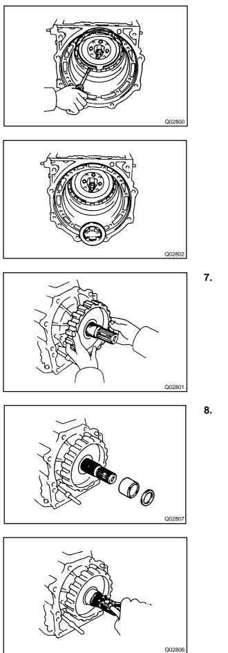
(g) Using a screwdriver, install the snap ring. HINT: Be sure the end of the snap ring is not aligned with the cutout portion of the transmission case.
