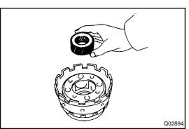
7. REMOVE REAR PLANETARY SUN GEAR Remove the sun gear from the rear planetary gear.
