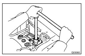
**REMOVE ONE-WAY CLUTCH RETAINER** 17.
