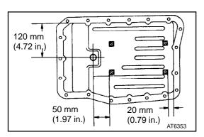
**36. INSTALL MAGNETS IN PAN** Install the 2 magnets in the oil pan.
