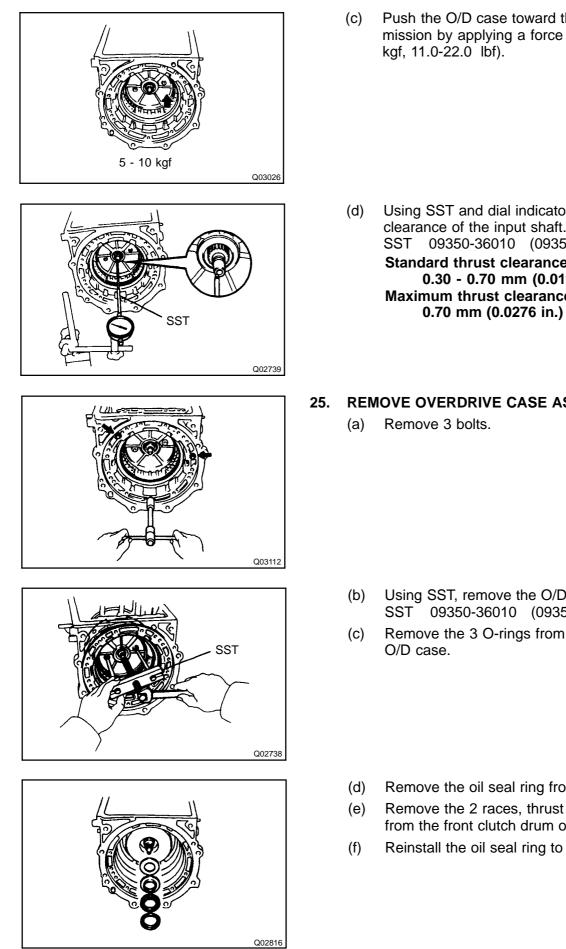
Push the O/D case toward the rear of the transmission by applying a force of 49 - 98 N (5 - 10
