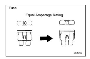
10. When replacing fuses, be sure the new fuse has the correct amperage rating. DO NOT exceed the rating or use one with a lower rating.
