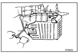
9. **REMOVE TRANSFER ASSEMBLY** Remove the 6 bolts and the transfer.
