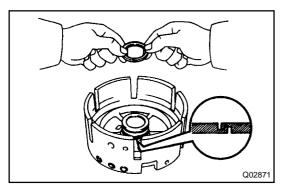
(c) Remove the piston return spring.
