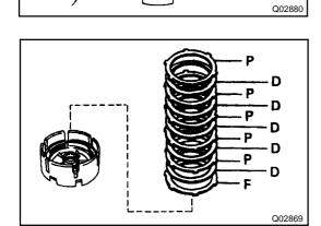
(b) Remove the flange, 5 discs end 5 plates.
