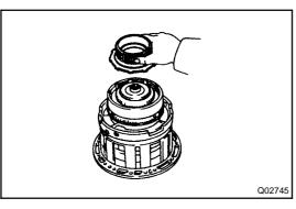
(c) Install the rear clutch hub onto the clutch drum.
