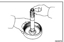
Coat a new oil seal ring with ATF, and install it on the intermediate shaft.
