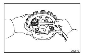
If the thrust clearance is greater than maximum, replace the planetary gear.
