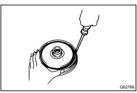
(b) Remove the flange, 3 discs and 3 plates.
