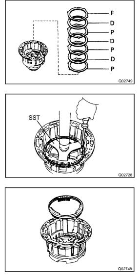
(b) Remove the flange, 3 discs and 3 plates.
