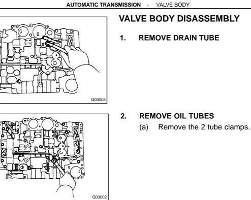
(b) Using a large screwdriver, pry out the 3 oil tubes.
