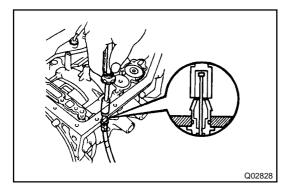
**REMOVE THROTTLE CABLE** 16. Using 10 mm socket driver, remove the throttle cable
