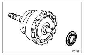
(b) Remove the output shaft from the rear planetary gear.
