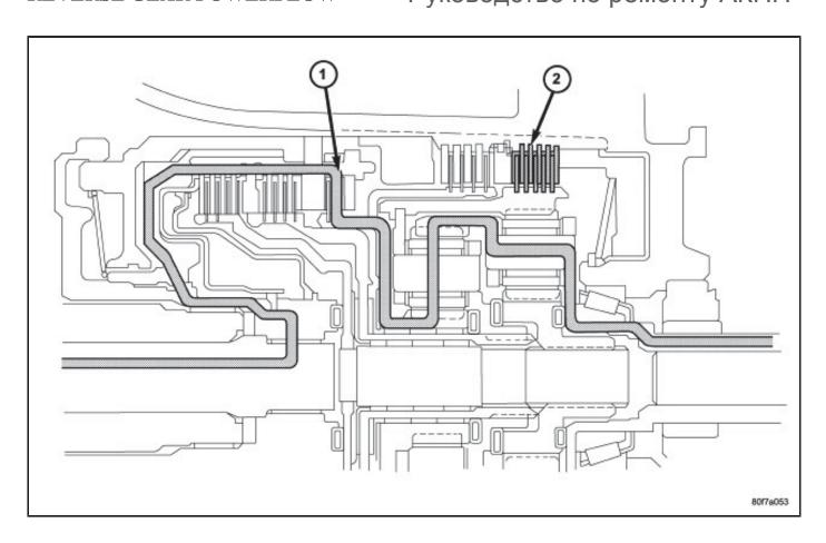
In reverse, input power is through the reverse clutch (1). When applied, the reverse clutch drives the front sun gear through the overdrive hub and shaft. The L/R clutch (2) is applied to hold the front carrier/rear annulus assembly stationary. The front carrier is being held by the L/R clutch so the pinions are forced to rotate the front annulus/rear carrier assembly in the reverse direction. Output torque is provided, in reverse, with a gear ratio of 2.21:1.
