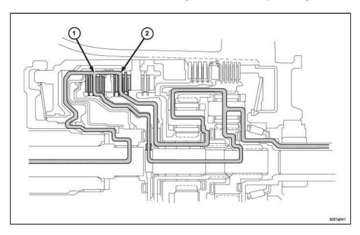
In third gear, two input clutches are applied to provide torque input: the underdrive clutch (1) and overdrive clutch (2). The underdrive clutch rotates the rear sun gear, while the overdrive clutch rotates the front carrier/rear annulus assembly. The result is two components (rear sun gear and rear annulus gear) rotating at the same speed and in the same direction. This effectively locks the entire planetary gearset together and is rotated as one unit. The gear ratio in third is 1:1.
